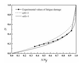
Fig. 1. Comparison among the experimental curve between fatigue damage - versus lifetime and the curves of literature models
