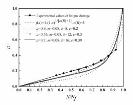
Fig. 3. Comparison among the theoretical curves between fatigue damage - versus lifetime based on equation (24) and the experimental curve
