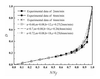
Fig. 4. Comparison among the theoretical curves between fatigue damage - versus lifetime based on equation (24) and the experimental curve
