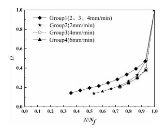
Fig. 5. Measured curves of the relationship between fatigue damage - versus lifetime of different loading rates
